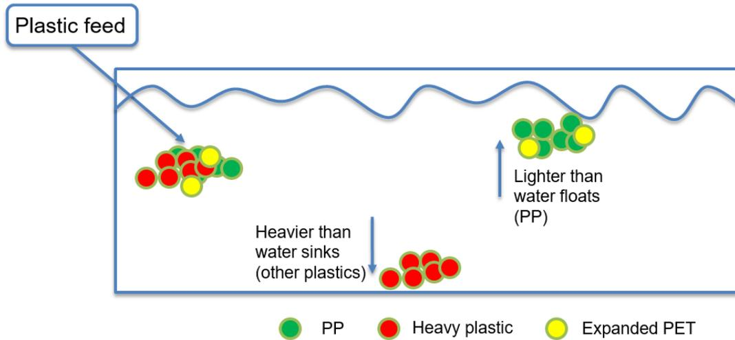
Figure 6 Sink/float process with mixed plastic contaminated with expanded PET
