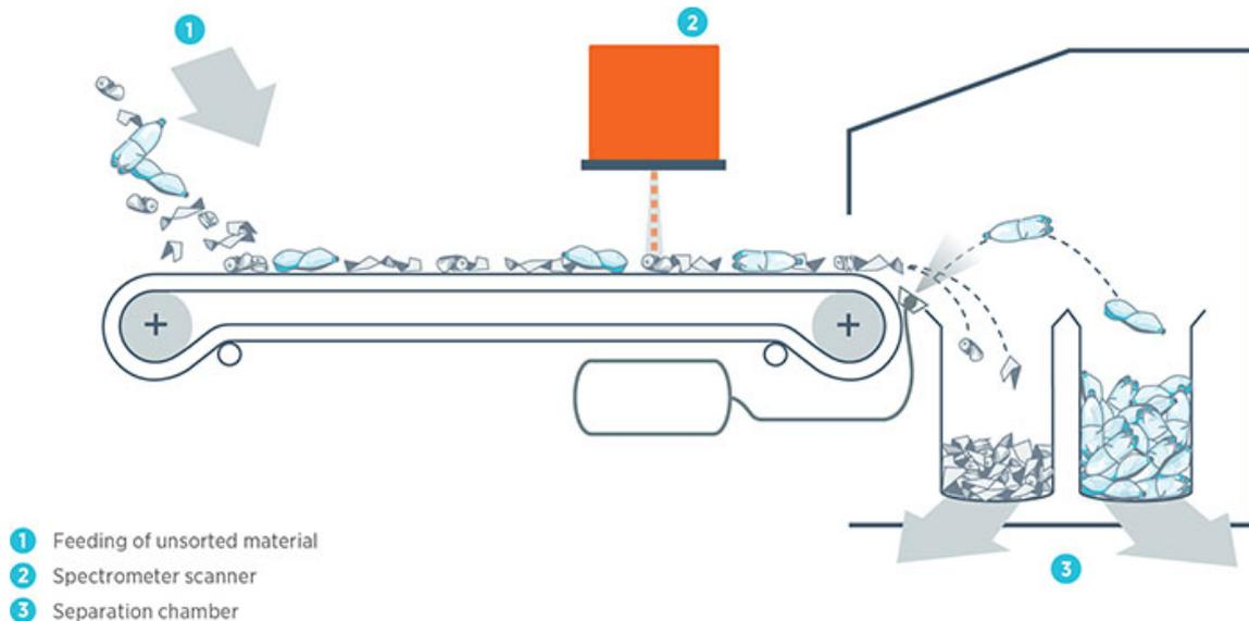
Figure 1 NIR sorter. In this example the blue bottles are being 'picked' and the grey material is going to the 'unseen' bin. Image copyright TOMRA.
