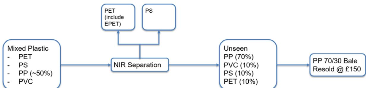
Figure 2 flow of a NIR system picking for PET and PS
