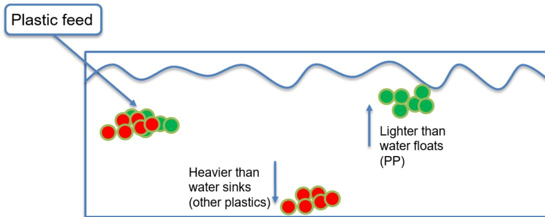
Figure 5 basic schematic of how a sink/float density separation process works
